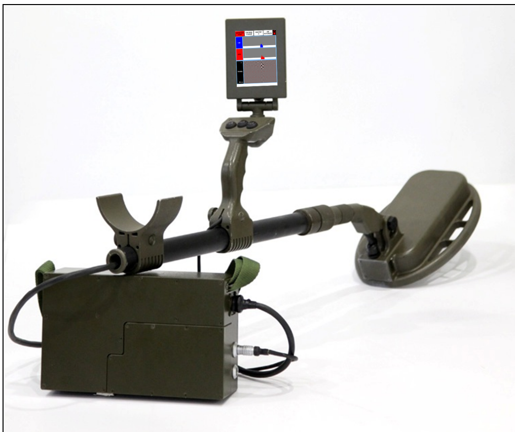
Figure-2 General view of dual sensor mine detection system (SEZER)
