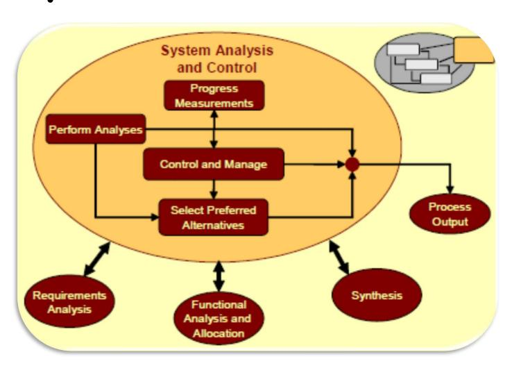
The system engineering process is the engine that ensures a balanced development of system products and sub-processes in each development step.
